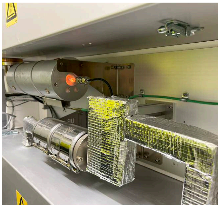
The \text{SO}_2 scrubber and the TRS converter between the two measurement cells. Note the red glow from the hot converter!
