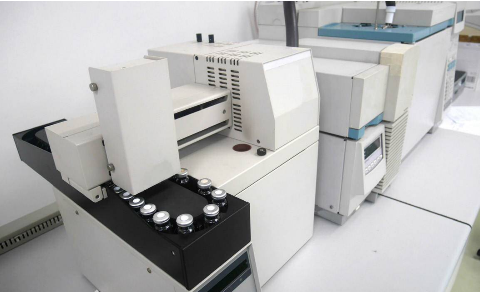
An example of a combined gas chromatograph and mass spectrometer (GC-MS) that could be used to analyse dioxins samples at a laboratory.
