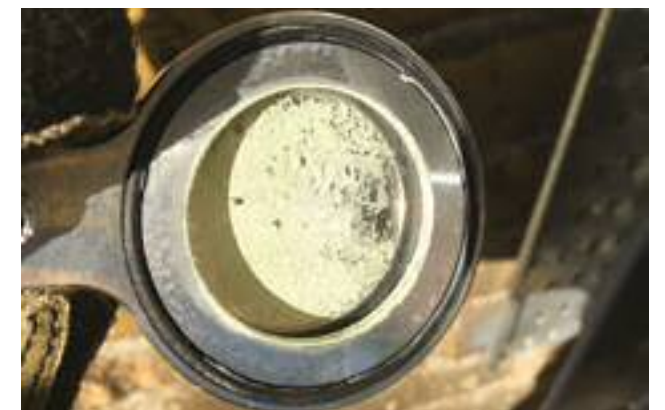
The reason why extractive systems are not suitable for this type of monitoring application. During the installation process of the OPSIS systems, the RE060s mounted on the gas ducts were temporarily without supply of purge air. The result is shown in the picture: rapid build-up of condensed sulfur and sulfuric salts on the window surface facing the flue gas. Imagine what will happen when sending such gas through extraction lines, valves and dilution units to a conventional SO 2 analyser! The monitoring paths now work fine with cleaned windows and proper supply of purge air.
