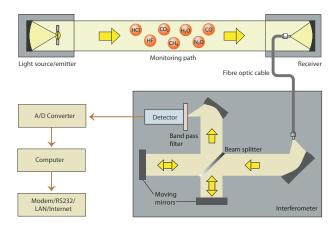
OPSIS has developed an analyser for monitoring compounds specifically in the infra-red wavelength range area. The OPSIS IR technique is based on the same method for identifying and measuring concentrations of various compounds as the comprehensive OPSIS spectrometer technique, described on the previous page.
