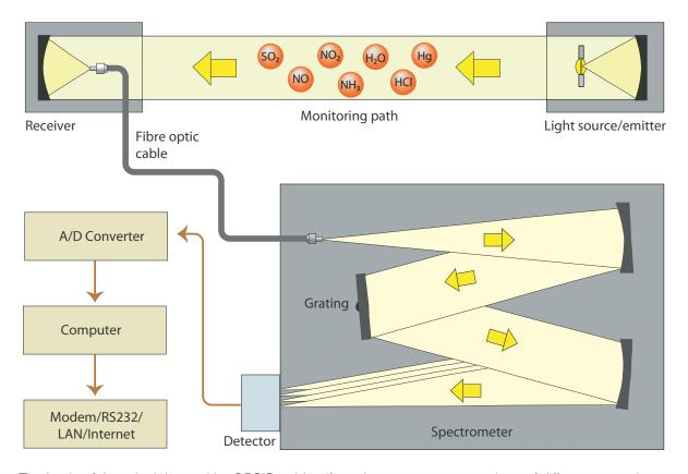
The basis of the principle used by OPSIS to identify and measure concentrations of different gases is scientifically well established: Differential Optical Absorption Spectroscopy (DOAS), which is based on Beer-Lambert's absorption law. It states the relationship between the quantity of light absorbed and the number of molecules in the lightpath.
