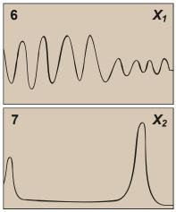
6-7. The gases that absorb light in this wavelength range are already known, and a pre-recorded reference spectrum for each gas is stored in the computer's memory. In this example there are only two gases, called  $X_1$  and  $X_2$ . The task is to determine the proportions of  $X_1$  and  $X_2$  that combine to give the best match for Z. The system achieves this by very rapidly creating a new curve out of the
