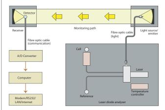
OPSIS LD500 laser diode gas analyser, based on the TDL (Tuneable Diode Laser) technique, emits laser light in the near infra-red section of the wavelength spectrum. The measurement is made by rapidly scanning the laser over the absorption line in the gas absorption spectrum.
