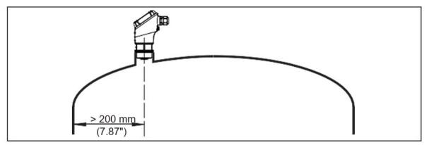
Fig. 4: Mounting the radar sensor on round vessel tops
