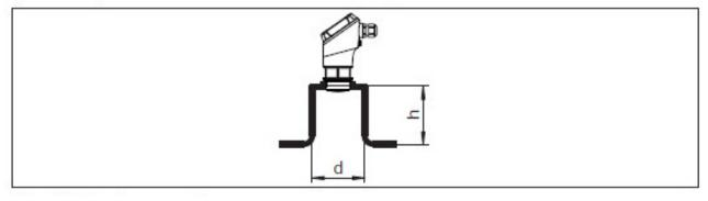
Fig. 8: Mounting the radar sensor with stand pipes
