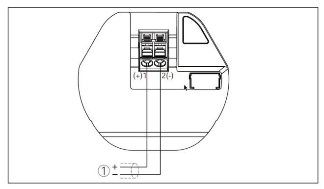
*Fig. 10: Connection compartment CNCR-210/220 1 Voltage supply +24 VDC, signal output*
