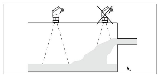
Fig. 7: Mounting the radar sensor with inflowing material
