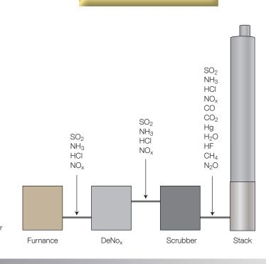
OPSIS monitoring system is an effective tool for controlling the different emissions and process control spots in a waste incinerator
