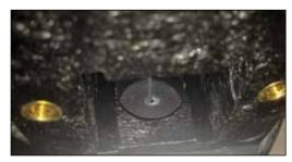
**Wiper Seal** — The new wiper seal completely wipes the cable clean before it retracts into the mechanical cavity of the SmartBob2 housing to prevent material from entering the device. It also helps seal the unit to eliminate any airborne particulates from entering the cavity while taking a measurement.
