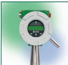
VorTek Instruments' Pro-V™ multivariable flowmeters utilize three primary sensing elements—a vortex shedding velocity sensor, an RTD temperature sensor, and a solid-state pressure transducer—to measure the mass flow rate of gases, liquids and steam.
