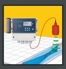
The NIVOSONAR GPA enables flow measurements on gravitational sewers, brook channels, irrigation channels or any other open channel with the help of a PARSHALL flume. The flume with EasyTREK integrated ultrasonic transmitter and MultiCONT process controller is able to create a complete flow-measurement system. The measuring flume is easy to install in new or existing channel structures.
